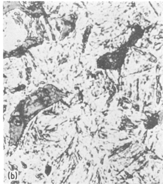
Figure 1 Microstructure of the sintered steels. (a) Typical microstructure of Ancoloy SA compact. Sintered, \times 1150 . (b) Microstructure of Ancoloy SA compact. Sintered, quenched and tempered, \times 1150 . (c) Ductile dimples in Ancoloy SA compact, \times 1790 .
